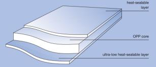
Treofan HLD is a biaxially oriented, co-extruded polypropylene film. Due to its ultra-low heat-seal threshold (below 80 °C), very high processing can be achieved. The film is corona-treated on one side to improve adhesion during printing and lamination. It has tailored and controlled slip properties to further enhance its high-speed running capabilities.
