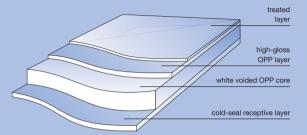
Treofan SHD is a biaxially oriented, co-extruded polypropylene film. The special external characteristics are the white colour produced by the compact cellular structure and the high gloss. Treofan SHD has been especially developed for cold-seal applications. The film is corona-treated on one side to improve the adhesion during printing and lamination.
