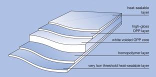
Treofan STD is a biaxially oriented, co-extruded polypropylene film. Its special characteristics are the white colour produced by the compact cellular structure and the low heat-sealing temperature on the inner layer. The film is corona-treated on one side to improve adhesion during printing and lamination.
