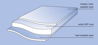
Treofan WSW is a white biaxially oriented, co-extruded polypropylene film. The special feature of Treofan WSW is the high whiteness. Treofan WSW is one-side treated to improve adhesion during printing and lamination.
